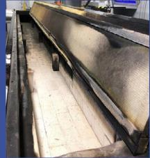
ASTM E84 is the standard test method for assessing the surface burning characteristics of building products to observe the flame spread and developed smoke density. The above photos show the STRONGIRT\* and mineral wool insulation assembly before (top) and after (bottom) testing.
